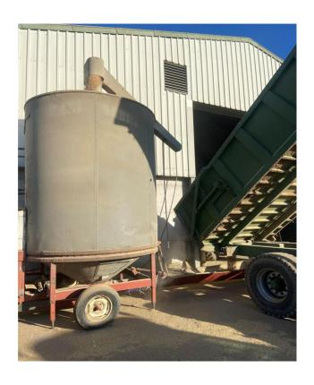
The next job has been drying the wheat grain from this years harvest before it is sold to the mill. The picture shows our mobile grain drier, which is a machine we rarely use, but thanks to our unusually wet and dull summer the wheat was harvested with a higher moisture content than they would accept without a price penalty, so it's well worth getting it out.
